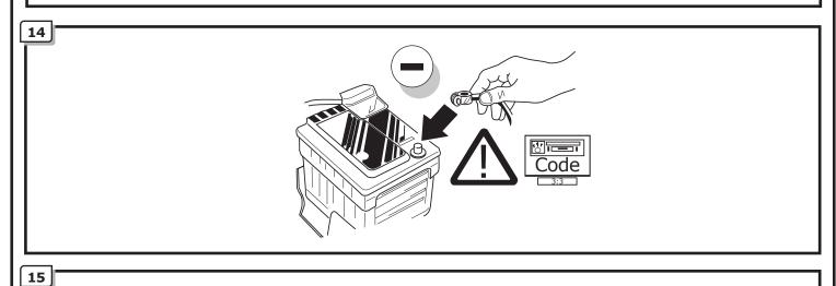
With a VAG Service tester with the help of SVM code '050200' the software of the vehicle must be adjusted to trailer coupling converted D12.
